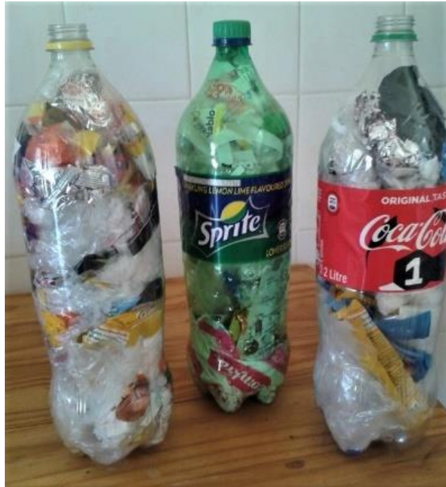
Figure 6.30 Eco-bricks under construction
